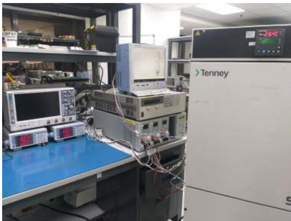
Figure 128 – Thermal Performance Set-up Using Thermal Chamber.
