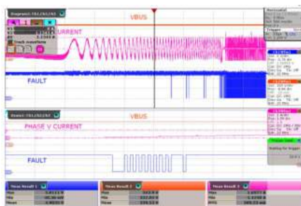
Figure 46 – OCP Fault Clear at R_{XL}/R_{XH} = 115 \text{ k}\Omega . CH2: V_{BUS} , 100 V / div. CH3: I_{PHASE} , 1 A / div. CH1: V_{FAULT} , 2 V / div. Time Scale: 500 ms / div. Time Scale (Zoomed Area): 100 \mu\text{s} / div. FAULT Clear = 0000000.
