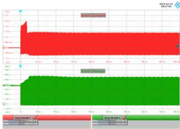
Figure 73 – 265 VAC, 42 V LED Load. Upper: I_{DRAIN} , 400 mA / div. Lower: V_{DRAIN} , 100 V / div., 40 ms / div.
