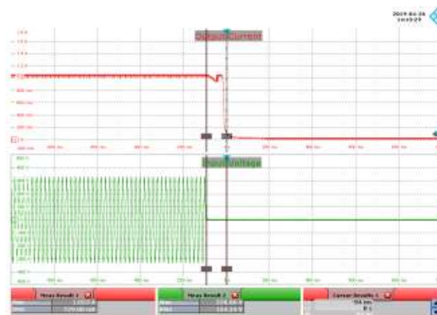
Figure 46 – 230 VAC, 42 V LED, Output Fall. Upper: I_{OUT} , 200 mA / div. Lower: V_{IN} , 100 V / div., 200 ms / div. Hold-up Time: 94ms.
