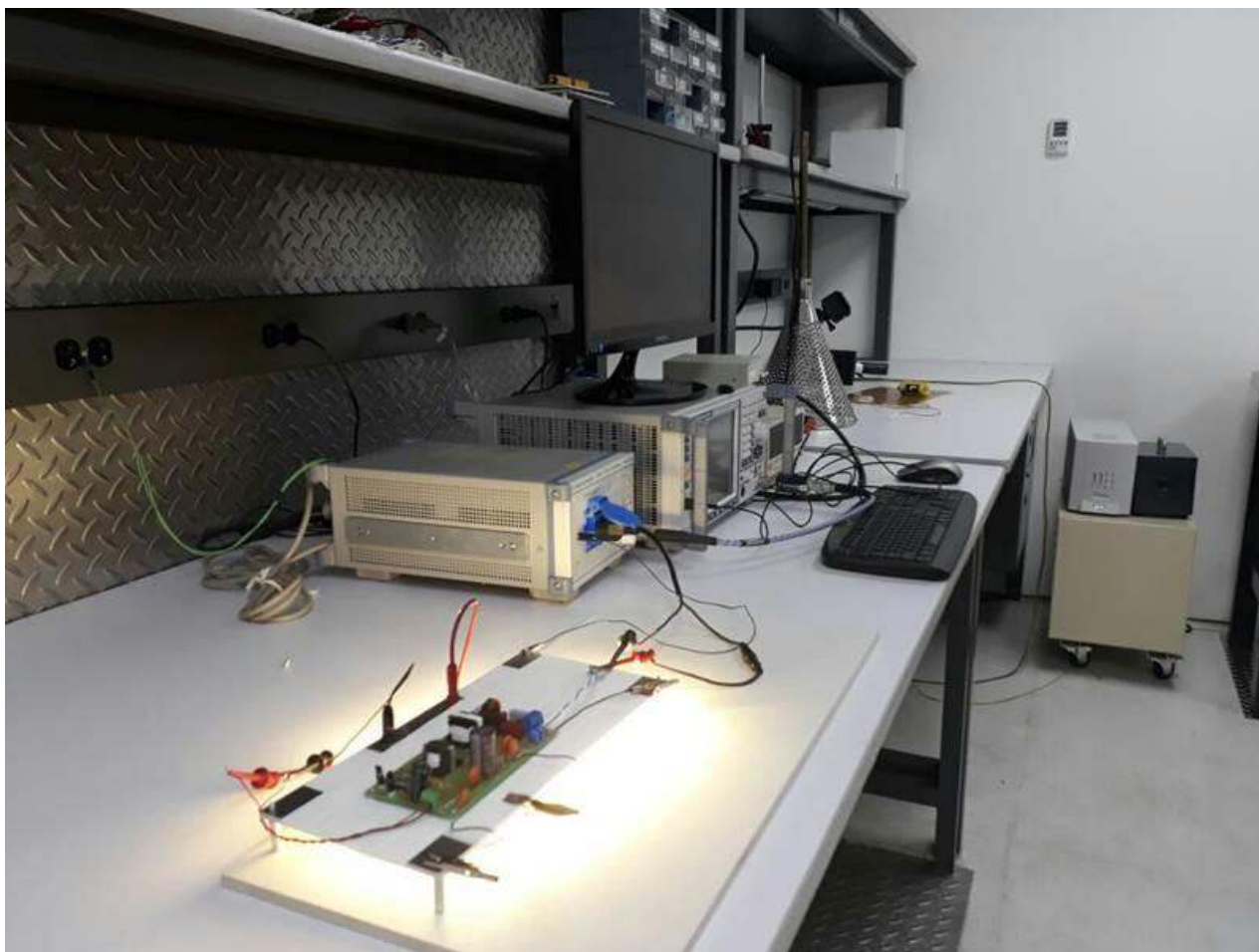
Figure 83 – Conducted EMI Test Set-up.
