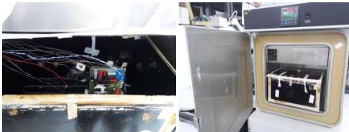
Figure 36 – Test Set-up Picture Thermal at 60 °C Ambient - Open Frame.
