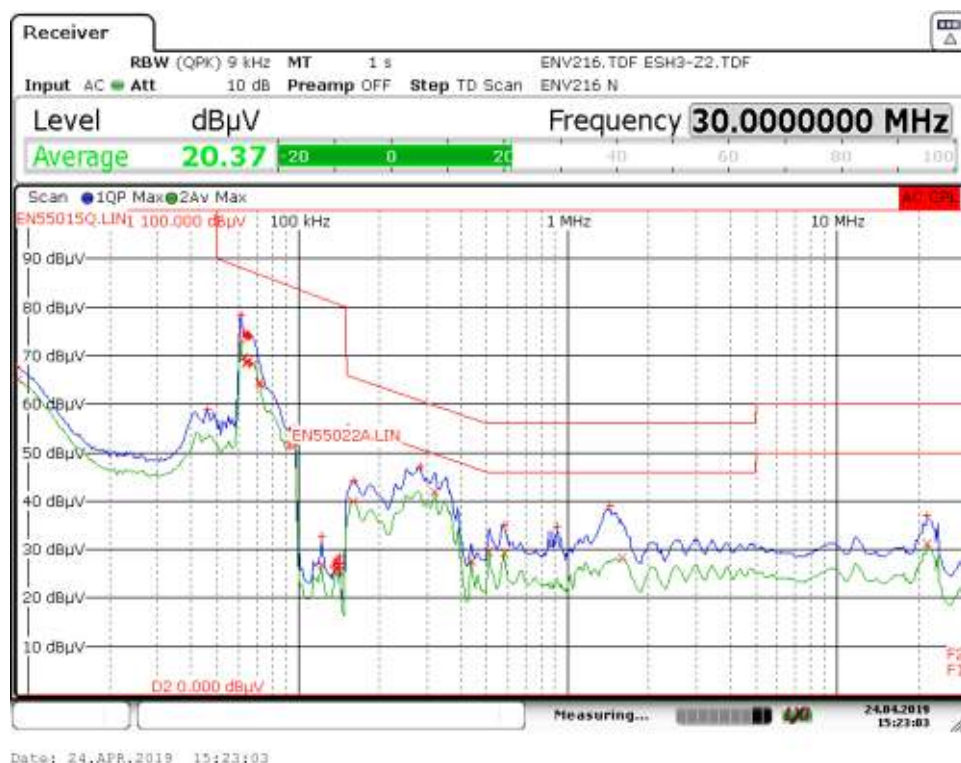
Figure 84 – Conducted EMI QP Scan at 42 V LED Load, 230 VAC, 60 Hz, and EN55015 B Limits.
