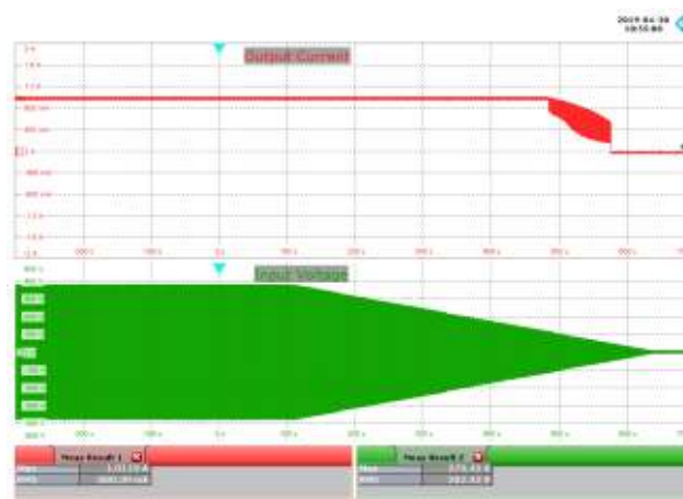
Figure 87 – Brown-out Test at 0.5 V / s Ch1: I_{OUT} , 400 mA / div. Ch2: V_{IN} , 100 V / div. Time Scale: 100 s / div.
