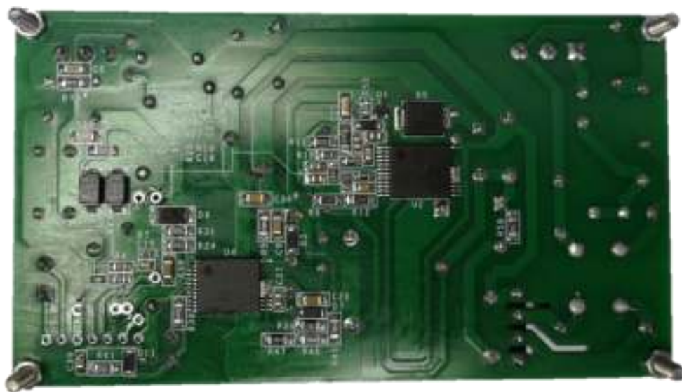
Figure 3 – Populated Circuit Board, Bottom View.
