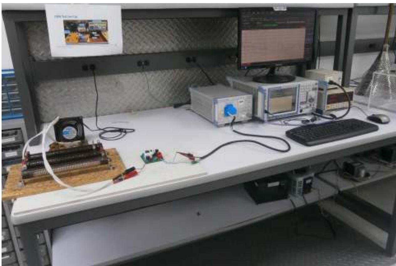
Figure 86 — Conducted EMI Test Set-up.
