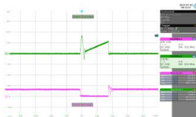
Figure 57 – 90 VAC 60 Hz, Output Shorted. Upper: I_{DRAIN} , 2 A / div. Lower: V_{DRAIN} , 200 V / div., 2 \mu s / div.
