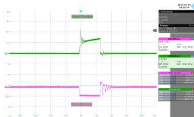
Figure 59 – 110 VAC 60 Hz, Output Shorted. Upper: I_{DRAIN} , 2 A / div. Lower: V_{DRAIN} , 200 V / div., 1 \mu s / div.
