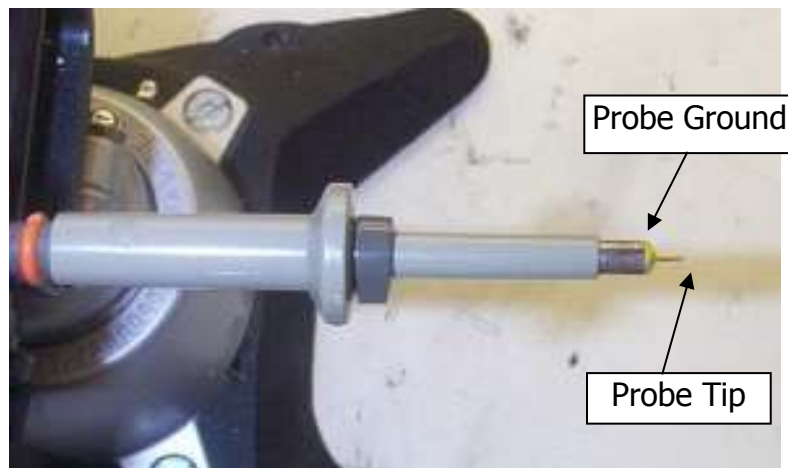
Figure 80 – Oscilloscope Probe Prepared for Ripple Measurement. (End Cap and Ground Lead Removed.)
