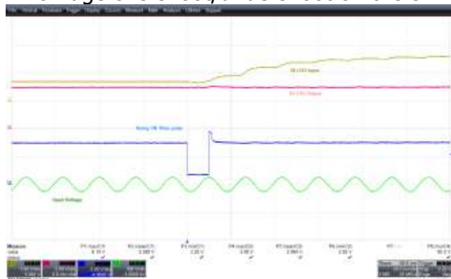
Figure 27 – Output Waveforms, 90 VAC, 60 Hz, Relay OFF to ON Transition. CH1: 3 V LDO Input. CH2: 3 V LDO Output. CH3: Relay ON Drive Pulse. CH4: Input AC Voltage.
