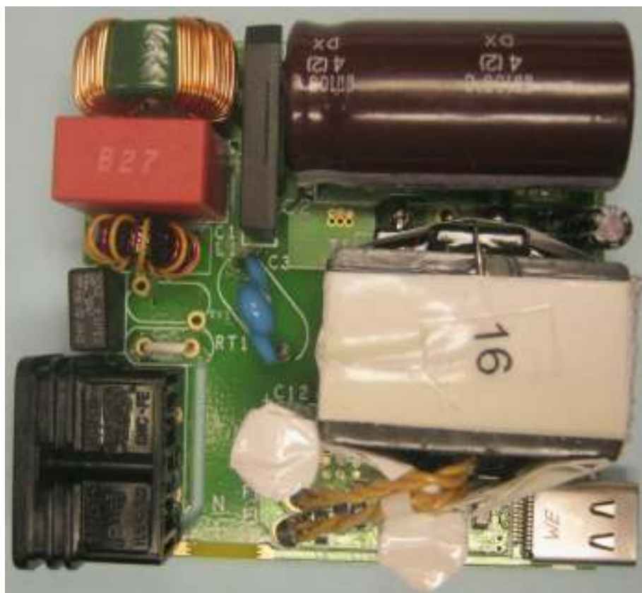
Figure 1 – Populated Circuit Board Photograph, Top.
