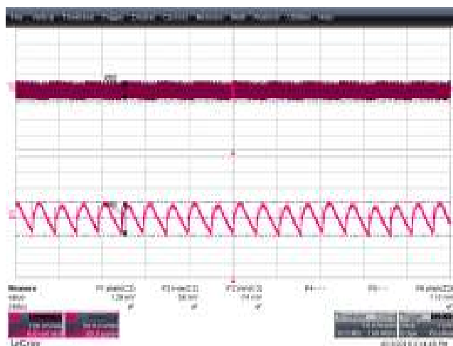
Figure 59 – Output Ripple.(pk-pk – 129 mV) 90 VAC Input, 9.0 V, 3 A Load. V_{OUT} , 100 mV / div., 10 ms / div.
