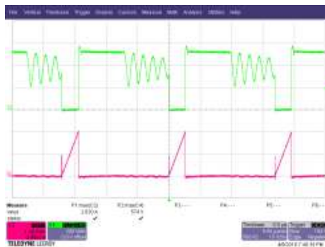
Figure 42 – Drain Voltage and Current Waveforms. 265 VAC, 9.0 V, 3 A Load, (574 V MAX ). Upper: V DRAIN , 200 V / div. Lower: I DRAIN , 1 A / div., 5 μs / div.
