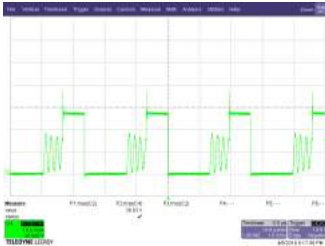
Figure 45 – SR FET Voltage Waveforms. 90 VAC, 9 V, 3 A Load, (36.83 V MAX ). C4: SR_V DRAIN , 10 V / div., 10 μs / div.
