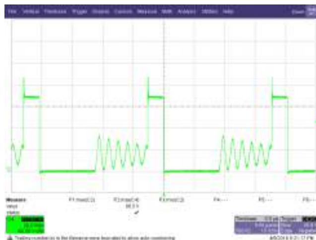
Figure 48 – SR FET Voltage Waveforms. 265 VAC, 15 V, 3 A Load, (86.5 V MAX ). C4: SR_V DRAIN , 20 V / div., 5 μs / div.
