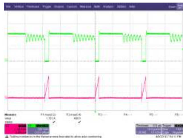
Figure 38 – Drain Voltage and Current Waveforms. 265 VAC, 9.0 V, 3 A Load, (489 V MAX ). Upper: V DRAIN , 200 V / div. Lower: I DRAIN , 1 A / div., 10 μs / div.
