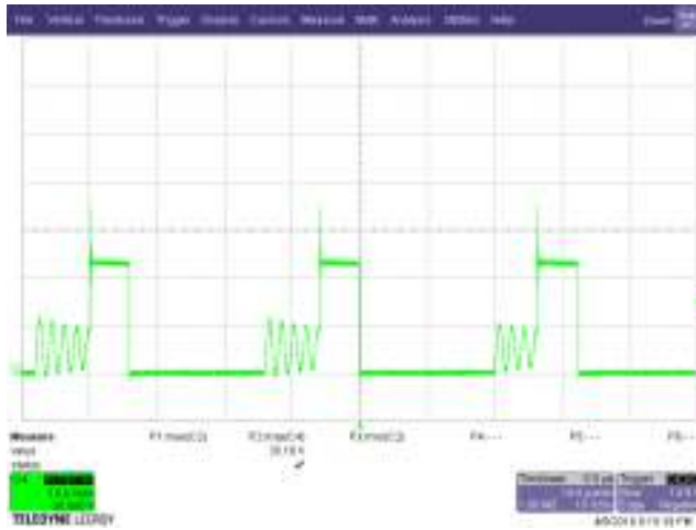
Figure 43 – SR FET Voltage Waveforms. 90 VAC, 5 V, 3 A Load, (35.16 V MAX ). C4: SR_V DRAIN , 10 V / div., 10 μs / div.
