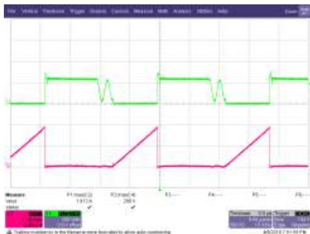
Figure 39 – Drain Voltage and Current Waveforms. 90 VAC, 15 V, 3 A Load, (298 V MAX ). Upper: V DRAIN , 200 V / div. Lower: I DRAIN , 1 A / div., 5 μs / div.
