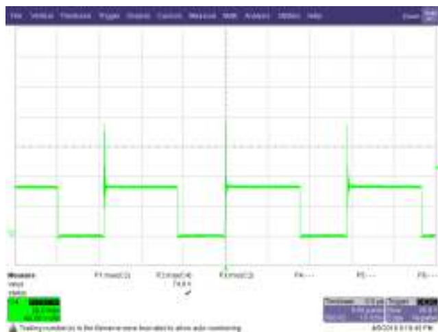
Figure 49 – SR FET Voltage Waveforms. 90 VAC, 20 V, 3 A Load, (74.8 V MAX ). C4: SR_V DRAIN , 20 V / div., 5 μs / div.
