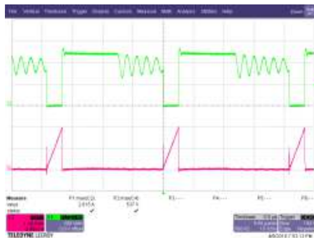
Figure 40 – Drain Voltage and Current Waveforms. 265 VAC, 15 V, 3 A Load, (537 V MAX ). Upper: V DRAIN , 200 V / div. Lower: I DRAIN , 1 A / div., 5 μs / div.
