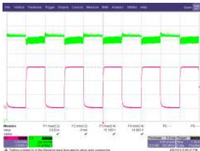
Figure 31 – Transient Response. 90 VAC, 15 V, 0 – 3 A Load Step. V_{MIN} : 14.983 V, V_{MAX} : 15.189 V. Upper: V_{OUT} , 0.2 V / div., 5 ms / div. Lower: I_{LOAD} , 1 A / div.
