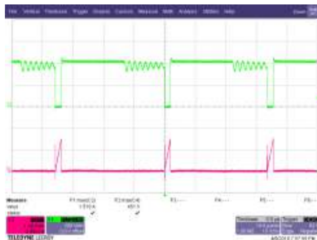
Figure 36 – Drain Voltage and Current Waveforms. 265 VAC, 5 V, 5 A Load, (451 V MAX ). Upper: V DRAIN , 200 V / div. Lower: I DRAIN , 1 A / div., 10 μs / div.
