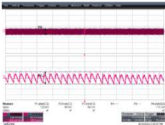
Figure 61 – Output Ripple.(pk-pk – 123 mV) 90 VAC Input, 15.0 V, 3 A Load. V_{OUT} , 100 mV / div., 10 ms / div.
