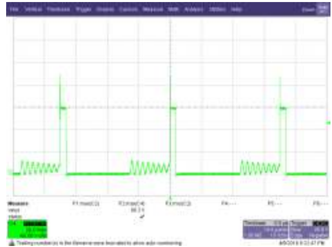
Figure 44 – SR FET Voltage Waveforms. 265 VAC, 5 V, 3 A Load, (88.3 V MAX ). C4: SR_V DRAIN , 20 V / div., 10 μs / div.
