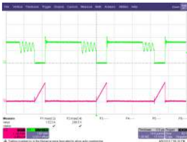
Figure 35 – Drain Voltage and Current Waveforms. 90 VAC, 5.0 V, 3 A Load, (209.5 V MAX ). Upper: V DRAIN , 100 V / div. Lower: I DRAIN , 1 A / div., 10 μs / div.
