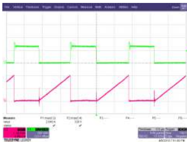
Figure 41 – Drain Voltage and Current Waveforms. 90 VAC, 20 V, 3 A Load, (328 V MAX ). Upper: V DRAIN , 200 V / div. Lower: I DRAIN , 1 A / div., 5 μs / div.
