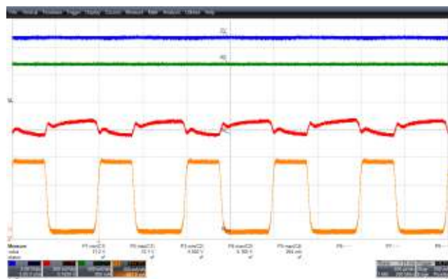
Figure 45 – Transient Response at 265 VAC, 50 Hz.
