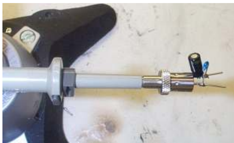
Figure 51 – Oscilloscope Probe with Probe Master ( www.probemaster.com ) 4987A BNC Adapter. (Modified with wires for ripple measurement, and two parallel decoupling capacitors added)
