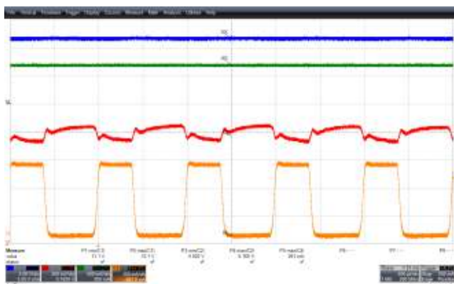
Figure 44 – Transient Response at 90 VAC, 60 Hz.
