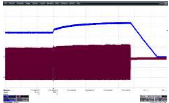
Figure 53 – 265 VAC 50 Hz, I_{OUT} = 1 A, OVP. Upper: V_{OUT} , 10 V / div., 5 s / div. Lower: Primary V_{DS} , 200 V / div. V_{OVP} = 34.4 V.
