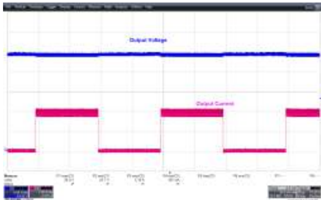
Figure 44 – 230 VAC 50 Hz, 0 A - 1.88 A Transient Load. Upper: V_{OUT} , 5 V / div. Lower: I_{OUT} , 1 A / div., 10 ms / div.
