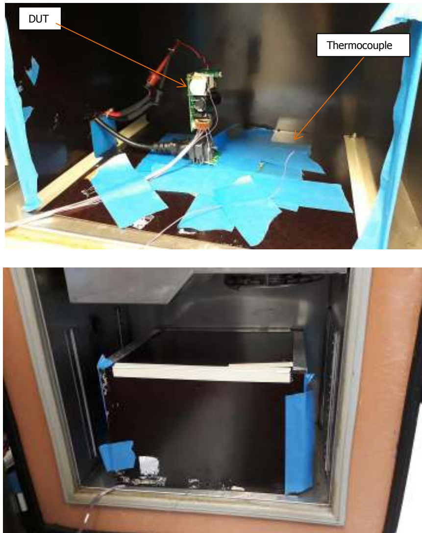
Figure 30 – Test Set-up Picture Thermal at 55 °C Ambient.
