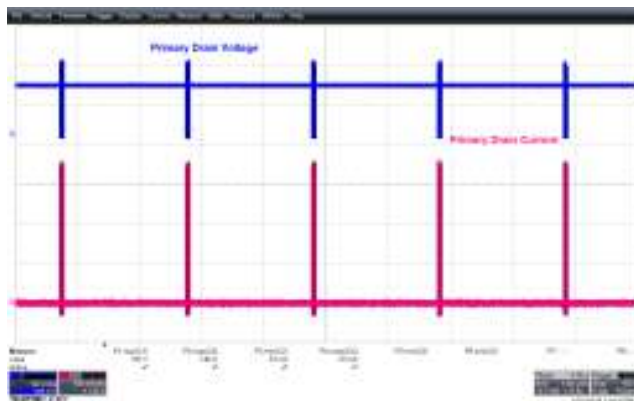
Figure 68 – 90 VAC 60 Hz, Output Shorted. Upper: I_{DRAIN} , 500 mA / div. Lower: V_{DRAIN} , 100 V / div., 1 s / div. I_{DS} = 1.82 A, V_{DS} = 193 V.
