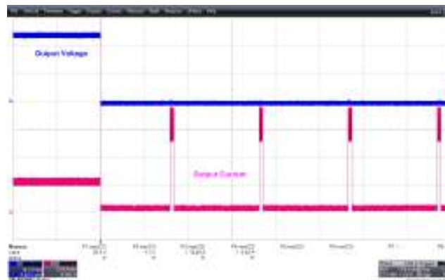
Figure 55 – 265 VAC 50 Hz, Full Load Short. Upper: V_{OUT} , 10 V / div., 1 s / div. Lower: I_{OUT} , 2 A / div.
