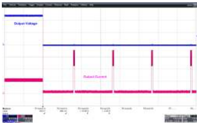
Figure 54 – 90 VAC 60 Hz, Full Load Short. Upper: V_{OUT} , 10 V / div., 1 s / div. Lower: I_{OUT} , 2 A / div.
