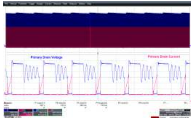
Figure 59 – 265 VAC 60 Hz, 24 V Full Load Normal. Upper: I_{DRAIN} , 500 mA / div. Lower: V_{DRAIN} , 100 V / div., 10 \mu s / div. I_{DS} = 1.83 A, V_{DS} = 592 V.
