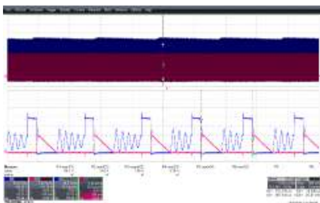
Figure 72 – 230 VAC 50 Hz, 24 V Full Load Normal. Upper: I_{DRAIN} , 5 A / div. Lower: V_{DRAIN} , 20 V / div., 10 \mu\text{s} / div. I_{DS} = 14\text{ A} , V_{DS} = 89.1\text{ V} .
