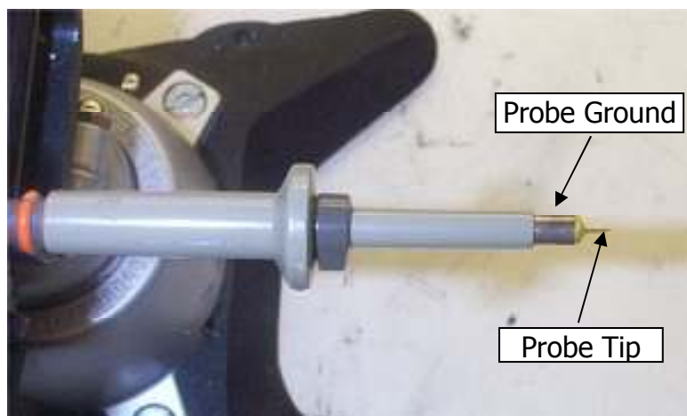
Figure 38 – Oscilloscope Probe Prepared for Ripple Measurement. (End Cap and Ground Lead Removed)
