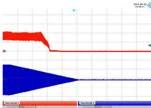
Figure 66 – Brown-out Test at 0.5 V / s. The Unit is Able to Operate Normally Without Any Failure and Without Flicker.
